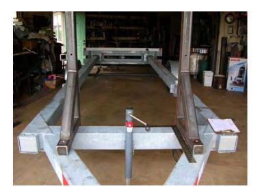
f. Project the hole locations to the opposite sides of the tubes. Make sure the holes are aligned and drill 7/8" diameter holes from each side of the tube.
