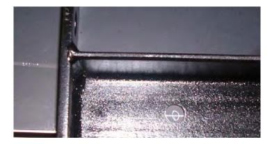
c. Mark the vertical position to place the edge of the bolt hole as close as practical to the bottom of the channel on the outside of the arrow board.
