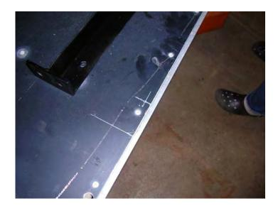
d. Center punch the hole positions and drill three 7/16" diameter holes in the arrow board, extending through both legs of the channel. Be careful to align the two holes in the channel legs.
