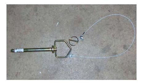
h. Using a pop rivet or metal screw attach the retaining pin using a ¼" clamp.
