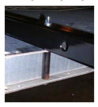
d. Identify if sign stand mounting holes are present in trailer A-frame. Four ¾" diameter holes in the trailer are required for mounting the sign stand. Two of the holes should be in the base of the A-frame, 11 inches from the inside of each burster tube. The other two holes should be in the top of the two upper A-frame tubes, approximately 17-7/8" from the base of the A-frame.
