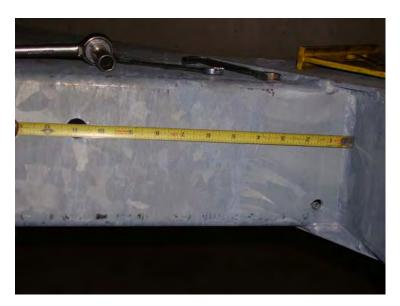
e. If the holes are present, skip to the next step. Otherwise, drill the missing holes. Place the lower sign support tubes on the trailer A-frame tongue. The centerline of each tube should be placed 11 in. from the inside of the adjacent burster tube. This positioning should place the centerlines of the two supports 36" apart. Make sure that the horizontal brace is perpendicular to the base of the A-frame. Mark the locations for the holes in the tubes.
