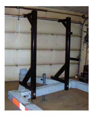
b. Attach cross braces (1"x1"x1/8" straps) between the lower sign support tubes using four ½"x4" grade 5 bolts, nuts, washers, and lock washers. Connect the two cross braces to each other using a ½"x1" grade 5 bolt, nut, washer, and lock washer.
