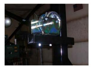
b. Unwind approximately 8 ft of ¼" diameter galvanized cable from the reel supplied. Cut the cable. Place one end of the cable through one of the access holes in the cable reel. Tape a small loop in the end of the cable. Secure the loop to the outside of the cable reel using the bolt and clamp supplied.
