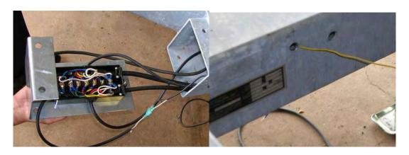
b. Push a 7/16" OD x 1/4" ID x 3/16" grove grommet onto the sign lead. Tape the string or wire to the conductor and pull it through to the burster tube.
