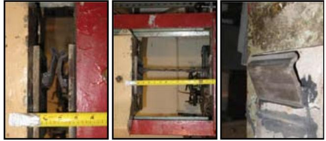
**Vertical Load** - Silicoflex was bonded to a concrete surface and filled with debris. A vertical load was placed on the Silicoflex seal, simulating how vehicular traffic would impact the joint. Silicoflex withstood 2,200 lbs of force without failing. It could have withstood more, but this was the capacity of the hydraulic actuator.
