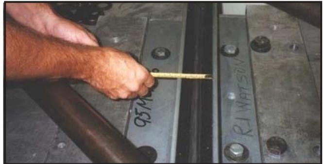
**Joint Debris** - Silicoflex was installed in a joint seal testing fixture, filled with debris, and then cycled to minimum and maximum openings. The inverted 'V' shape directs debris to the seal where it is bonded and fixed. This consequently causes debris to be channeled upwards, rather than staying trapped in the joint and overstressing the seal.
